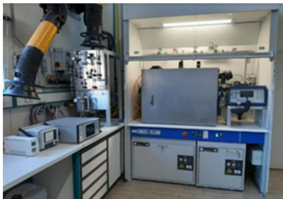
**Fig. 6: The online conditioning and analysis system of the methanol synthesis test plant at AL.**
